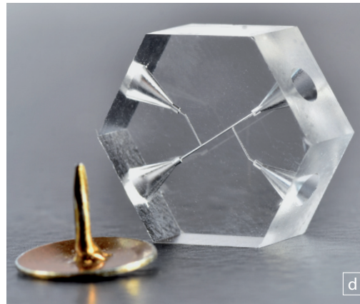
a A cell sorter for quicker antibiotic resistance test is being developed in cooperation with the group of Clinical Diagnostics from Fraunhofer ILT
