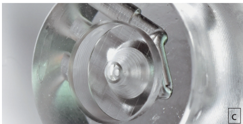
d A microfluidic chip for more efficient coupling of capillaries in capillary electrophoresis (cooperation with group of Analytical Chemistry at University of Tübingen)
